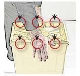
A sound ensures that the clip has been correctly inserted and the clip can be seen in the edge of the lid
