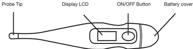
1. Remove the thermometer from the Storage Case. Press the On/Off Button to turn on the thermometer. All symbols will appear on the Display Window, indicating that the thermometer is functioning properly.
